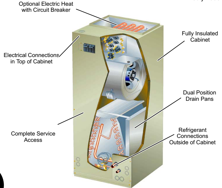
CB28UH Up-flow Position (With Optional Electric Heat)
