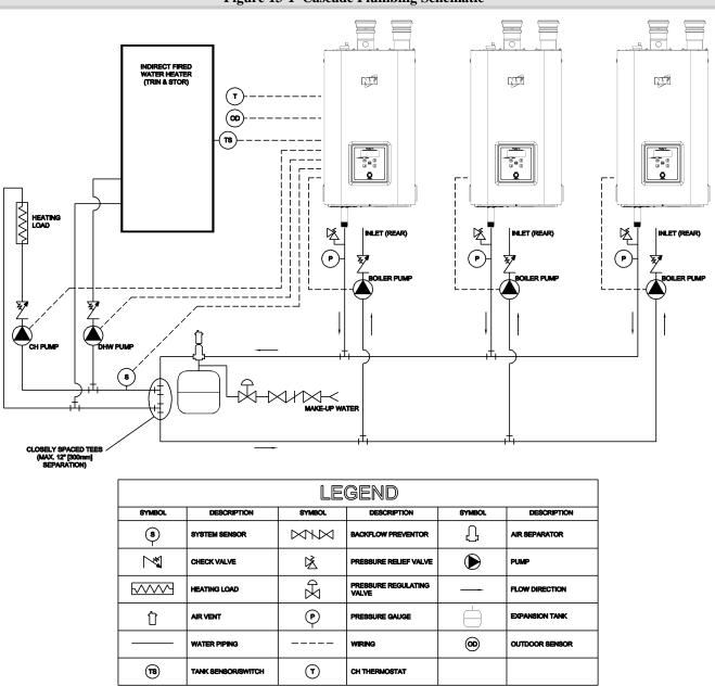
Figure 13-1 Cascade Plumbing Schematic
