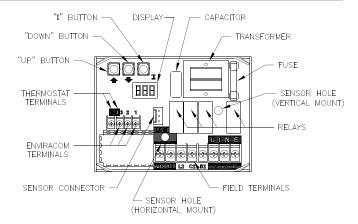
Figure 30: Intelligent Oil Boiler Control
