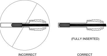
Figure 11: Limit Sensor Insertion
