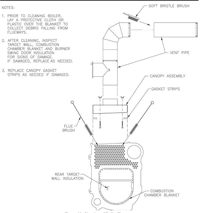
Figure 32: Cleaning of Boiler Flueways
