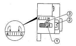
Figure 8: Riello Turbulator Setting
