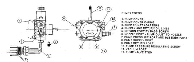
Figure 9: Riello Pump Connections and Port Identification
