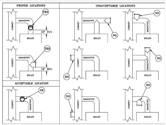
Figure 18: Proper and Improper Locations of Draft Regulator
