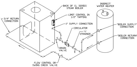
Figure 16: Indirect Water Heater Piping on CL Series Steam Boiler
