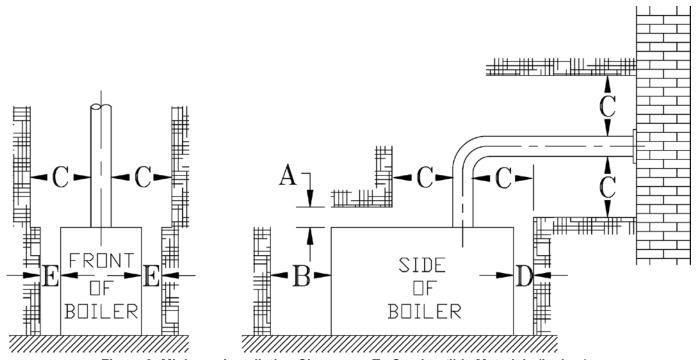
Figure 3: Minimum Installation Clearances To Combustible Materials (Inches)
