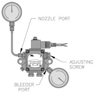
Figure 26: Adjusting Fuel Pump Pressure
