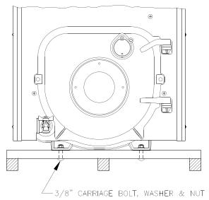
Figure 4: Removal of Boiler From Skid
