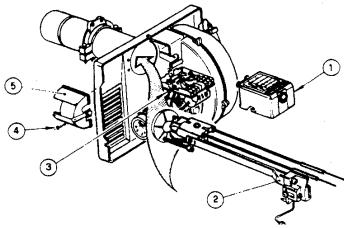
Figure 5: Installation/Removal of Riello Drawer Assembly
