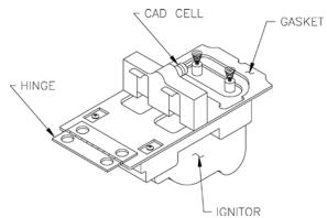
Figure 28: Cad Cell Location
