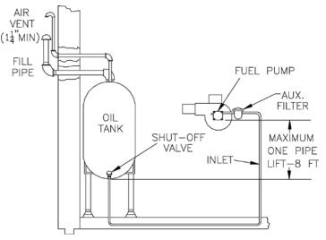
Figure 19: Single Pipe Oil Line
