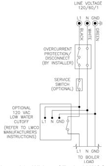
Figure A2: Wiring of Typical LWCO
