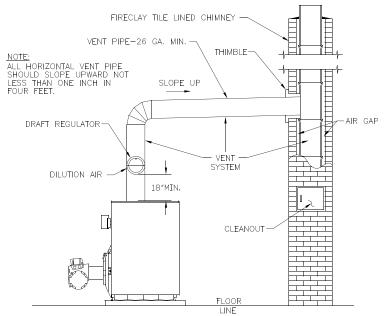
Figure 17: Recommended Smokepipe Arrangement and Chimney Requirements
