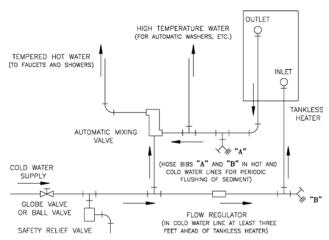
Figure 15: Schematic Tankless Heater Piping
