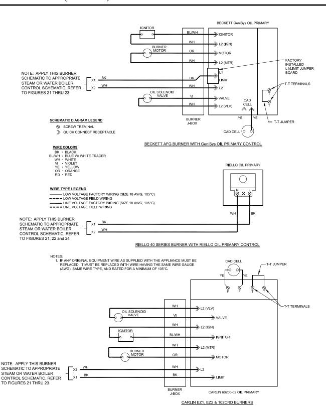
Figure 25: Schematic Wiring Diagrams For All Burner Options w/Various Oil Primary Controls
