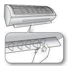
Move the blade left or right to keep the air flow direction in a constant position you prefer.
