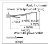
2. Insert both sides of core wire of the power cable into the connection sleeve.
