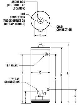
Maximum Hydrostatic Working Pressure: 150 PSI
