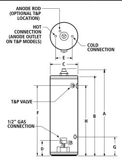
Maximum Hydrostatic Working Pressure: 150 PSI
