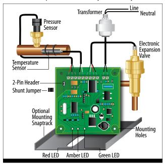
The KE2 Simple Superheat provides OEM customers a cost effective option for controlling Electronic Expansion Valves (EEV) for the best control possible. The controller is equipped with all necessary components for controlling the superheat, and can be configured to meet individual system needs. The controller also limits the OEMs exposure to field issues by preventing modifications by unauthorized personnel, eliminating nuisance trouble calls caused by improper field adjustments.
