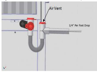
**Note:** Connect the drain through the trap to the condensation drain system in conformance to local plumbing codes.
