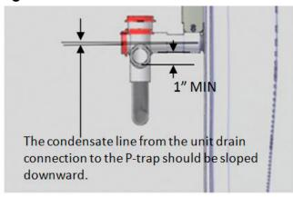
Figure 9b: Condensation Drain Drop
