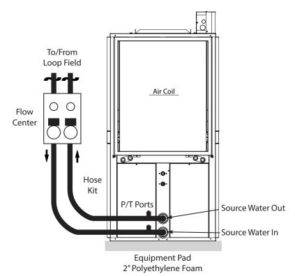
**Note:** P/T ports should be angled away from the unit for ease of gauge reading.
