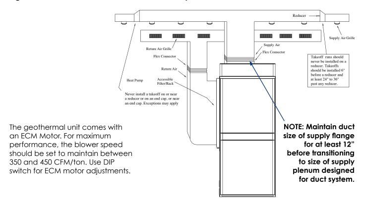
Figure 4: Ductwork with Split Damper Connection Setup
