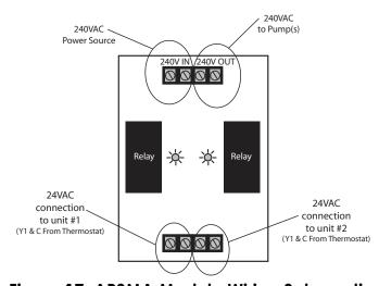
Figure 17: APSMA Module Wiring Schematic
