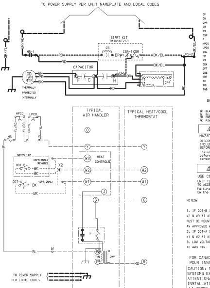
COMPRESSOR RUN CAPACITOR STARTING CAPACITOR CAPACITOR SWITCHING RELAY INDOOR FAN RELAY HIGH PRESSURE CUTOUT SWITCH LOW PRESSURE CUTOUT SWITCH INTERNAL OVERLOAD PROTECTOR SYSTEM ON-OFF SWITCH COMPRESSOR MOTOR CONTACTOR OUTDOOR ANTICIPATOR OUTDOOR FAN THERMOSTAT OUTDOOR TEMPERATURE SENSOR
