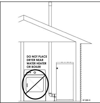
Figure 18 - Do Not Place Appliance Near Dryer
