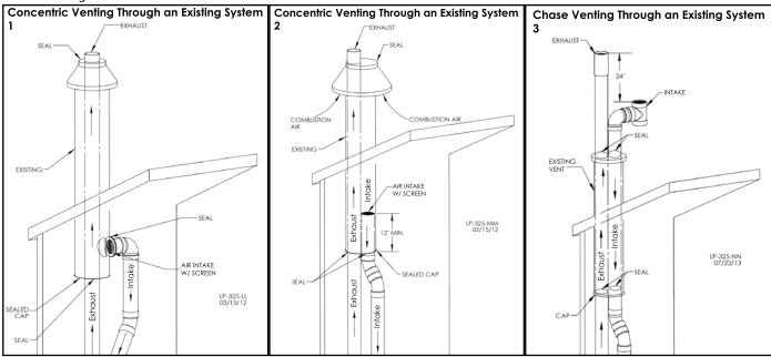
Figure 17 - 1, 2 - Concentric Venting Through an Existing System, 3, Chase Venting Through an Existing System
