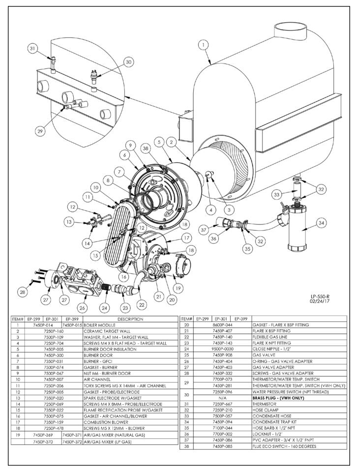
Figure 31 - Combustion System Replacement Parts - 299 - 399kBTU Models
