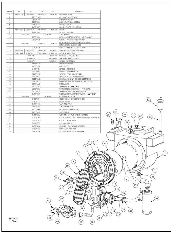
Figure 30 - Combustion System Replacement Parts - 80 - 220kBTU Models
