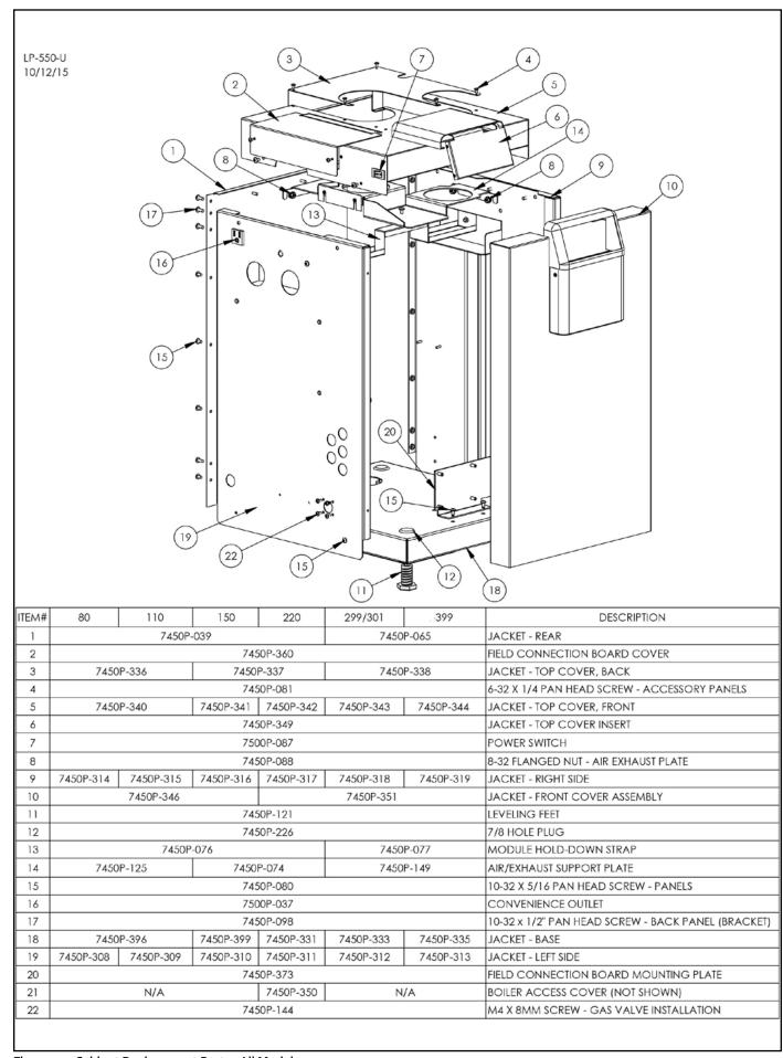
Figure 32 - Cabinet Replacement Parts - All Models
