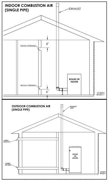
Figure 19 - Indoor and Outdoor Combustion Air - Single Pipe
