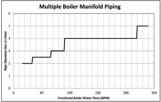
Figure 6 - Multiple Boiler Manifold Piping
