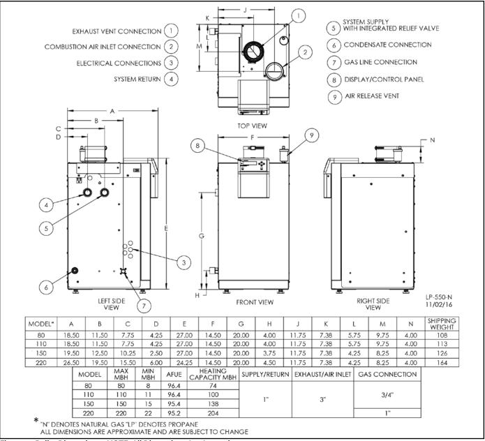
Figure 4 - Boiler Dimensions - NOTE: All Dimensions Are Approximate
