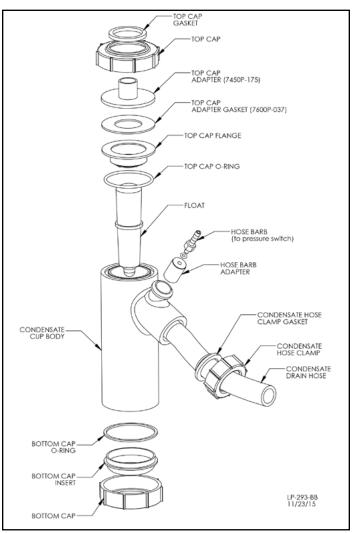
Figure 29 - Condensate Detail
