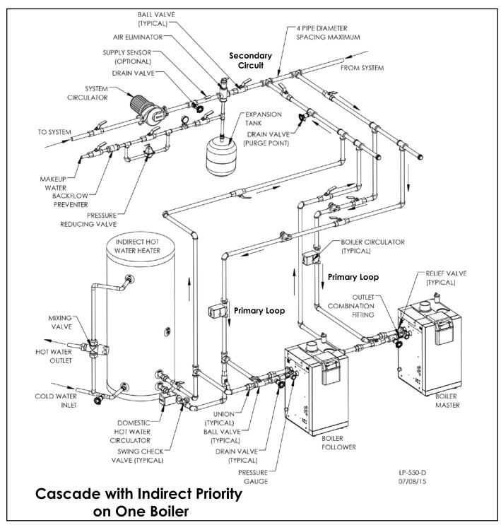
Figure 8 - Cascaded Boilers with Indirect Priority on a Single Boiler NOTES:
