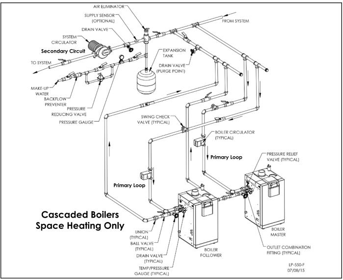
Figure 10 - Cascaded Space Heating
