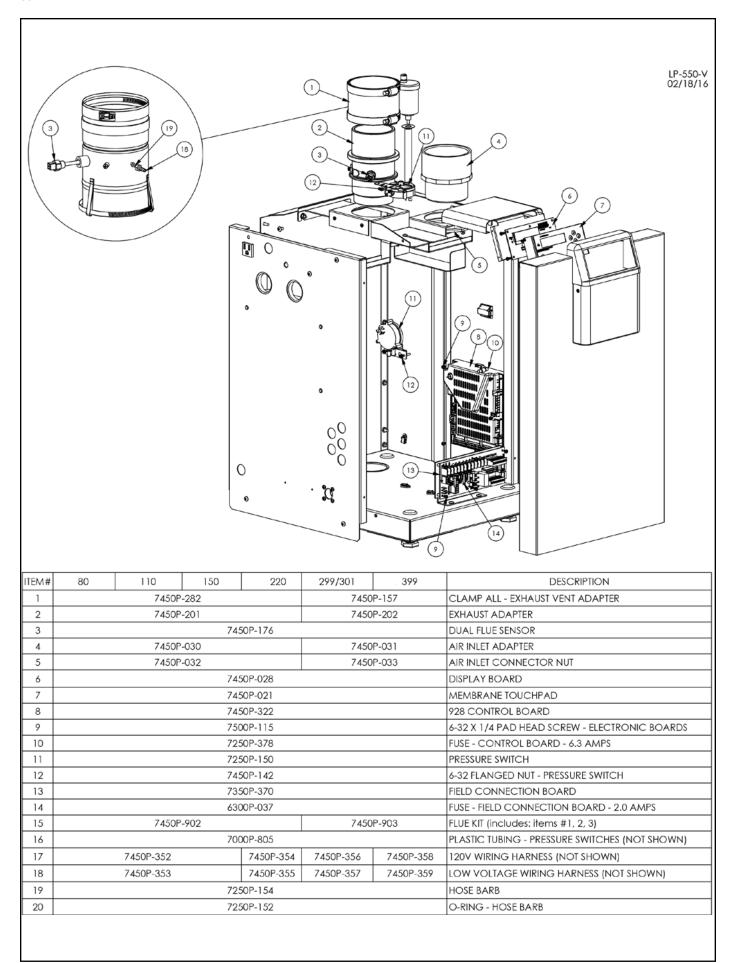
Figure 33 - Cabinet Replacement Parts - All Models
