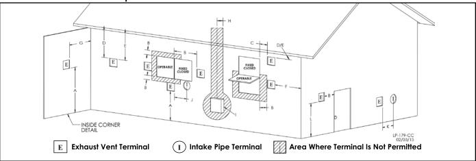
Figure 11 - Exit Terminals for Direct Vent Systems - ANSI Z223.1 / NFPA 54 for US and CAN/CSA B149.1 for Canada
