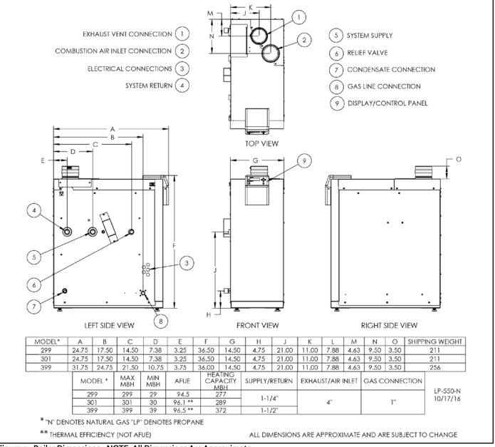
Figure 5 - Boiler Dimensions - NOTE: All Dimensions Are Approximate
