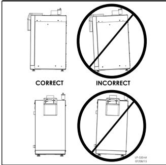
Figure 1 - Correct and Incorrect Leveling
