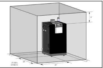
Figure 2 - Recommended Service Clearances
