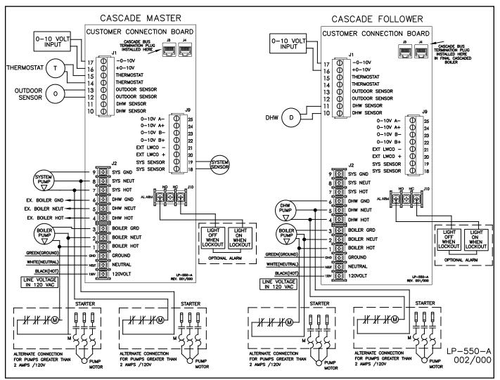
Figure 24 - Cascade Master and Follower Wiring
