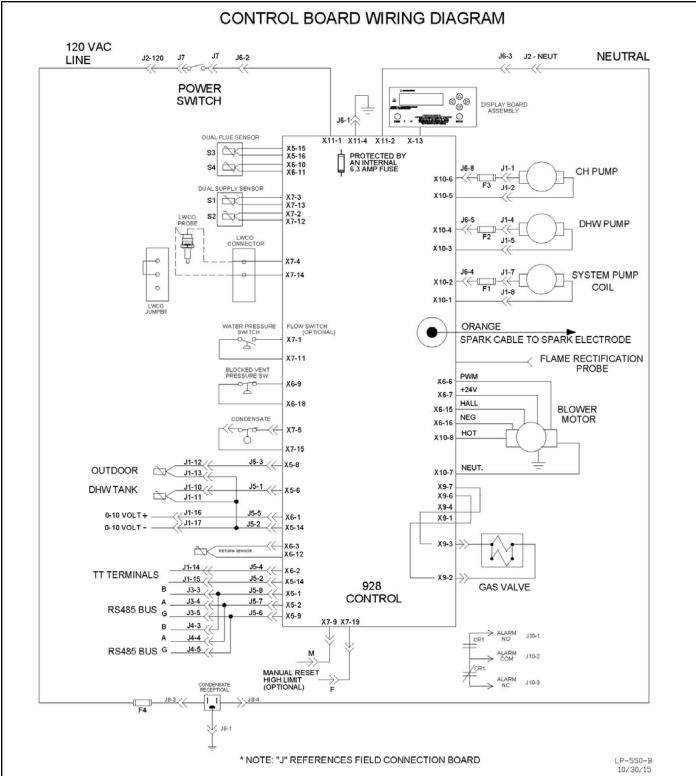
Figure 25 - Internal Connection Diagram
