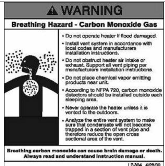
Figure 5 - CO Warning Label
