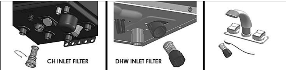
Figure 56 – Cleaning the Inlet Filter
