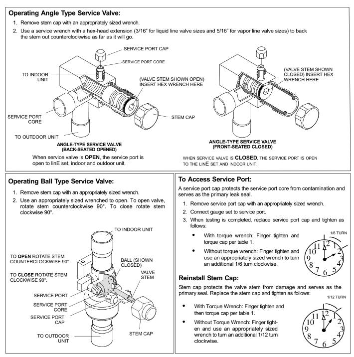
NOTE — A label with specific torque requirements may be affixed to the stem cap. If the label is present, use the specified torque.
