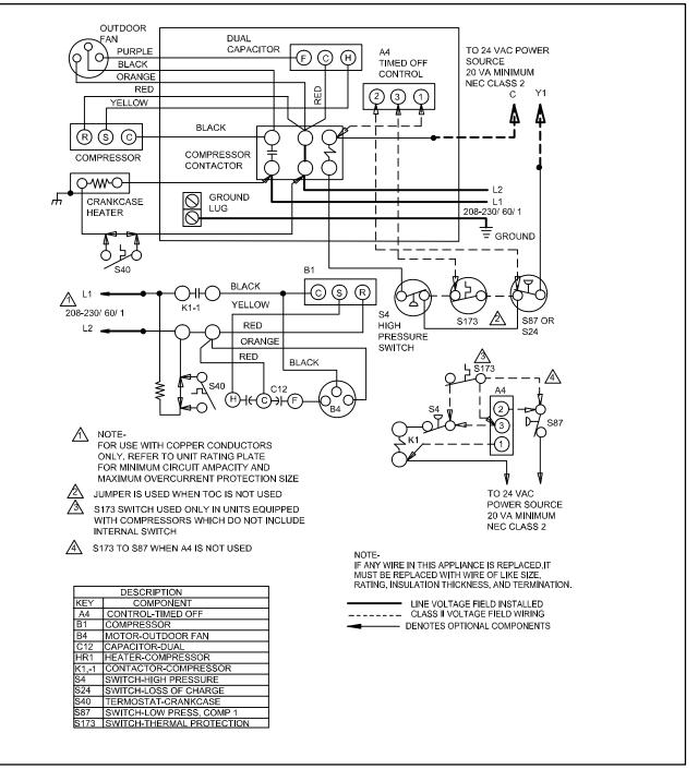
Figure 17. Typical Unit Wiring Diagram
