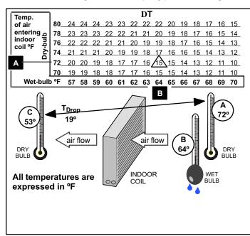
**1. Determine the desired DT**—Measure entering air temperature using dry bulb (**A**) and wet bulb (**B**). **DT** is the intersecting value of **A** and **B** in the table (see triangle).
