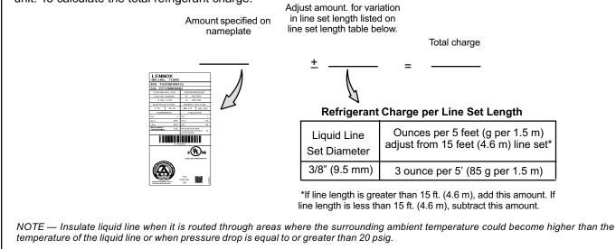
NOTE — The above nameplate is for illustration purposes only. Go to actual nameplate on outdoor unit for charge information.
