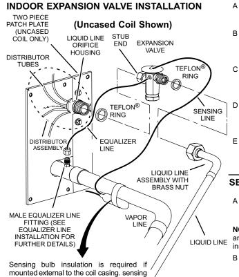
bulb installation for bulb positioning.
