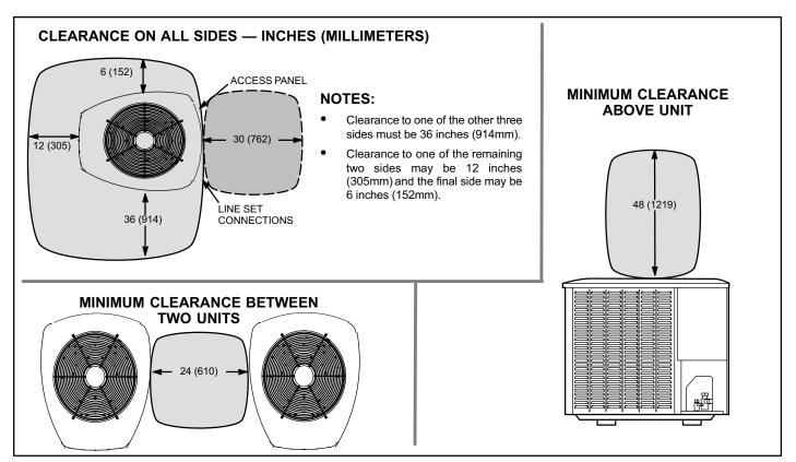
Figure 4. Installation Clearances
