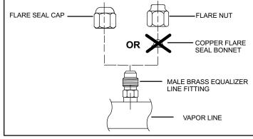
See the Lennox XC14 Engineering Handbook for approved expansion valve kit match-ups. The expansion valve unit can be installed internal or external to the indoor coil. In applications where an uncased coil is being installed in a field-provided plenum, install the expansion valve in a manner that will provide access for field servicing of the expansion valve. Refer to below illustration for reference during installation of expansion valve unit.
