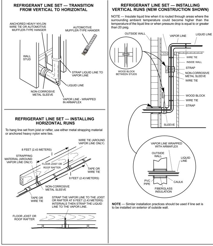
Figure 7. Line Set Installation
