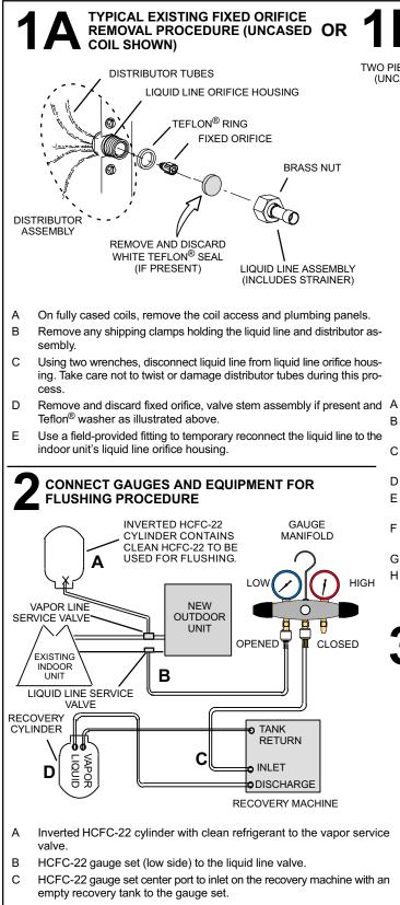
D Connect recovery tank to recovery machines per machine instructions.
