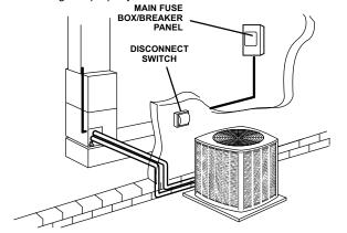
NOTE — Units are approved for use only with copper conductors. Ground unit at disconnect switch or to an earth ground. temperatures and pressures present during operation of an air conditioning system. Non-condensables and water suction combine with refrigerant to produce substances that corrode copper piping and compressor parts.
