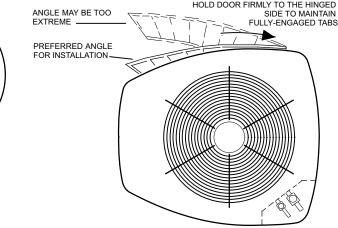
Figure 6. Removing and Installing Panels
