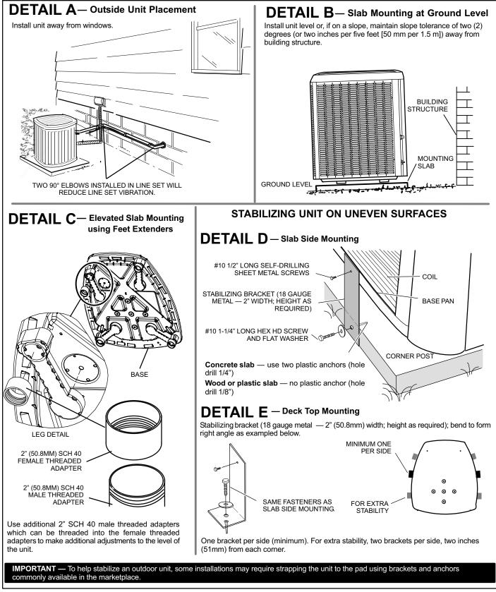
Figure 5. Placement, Slab Mounting and Stabilizing Unit
