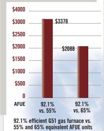
This chart depicts potential energy savings you can expect from the G51 gas furnace versus older furnaces with lower efficiency ratings. Criteria used in this example are 2,000 full-load heating hours, with a 60,000-Btuh heating design load and \$1.281 ccf for gas. Your actual savings will vary depending on the weather, local fuel rates and your lifestyle.
