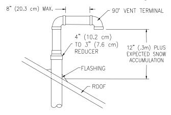
NOTE: For installations requiring both horizontal and vertical runs, the following rule must be followed: Total length of straight pipe (both horizontally and vertically) must not exceed the allowable length listed in the "Through The Wall" section of the table for total number of elbows used.
