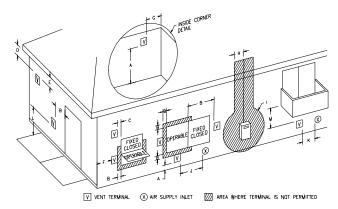
**Figure 1 - Vent Terminal Clearances**
