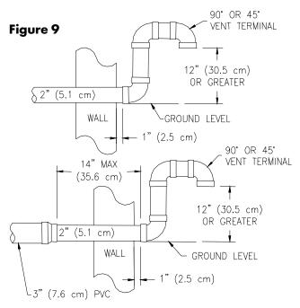
NOTE: For installations requiring both horizontal and vertical runs, the following rule must be followed: Total length of straight pipe (both horizontally and vertically) must not exceed the allowable length listed in the Table 7 and 8 for total number of elbows used.
