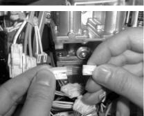
Connect the 2 pin connector from Communication Cable A into the 2 pin connector marked "MS".
