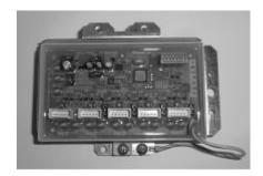
Remove the screw from the sheet metal reinforcement plate located at the bottom of the water heater cabinet, and then use it to secure the Master Communication PCB to the water heater cabinet.
