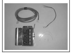
MSA-2S - Pack B Manifold Electronic Control System (For wiring Units 3, 4, and 5)
