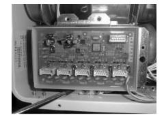
Connect the 5 pin connector from Communication Cable A (18 inch cable) to socket No. 1 on Master Communication PCR
