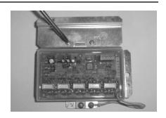
P.) Remove and discard sheet metal bracket leaving Master Communication PCB.
