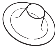
12 flat roof flashing
