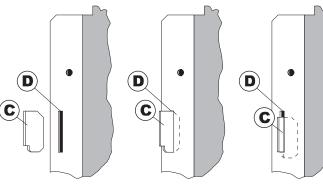
13. Open the small hinged panels on the top and bottom of the plastic side trims. Remove the retaining clips and discard. Slide the front panel upwards in the slots () and fasten in place using the screws (8) and washers (1).
