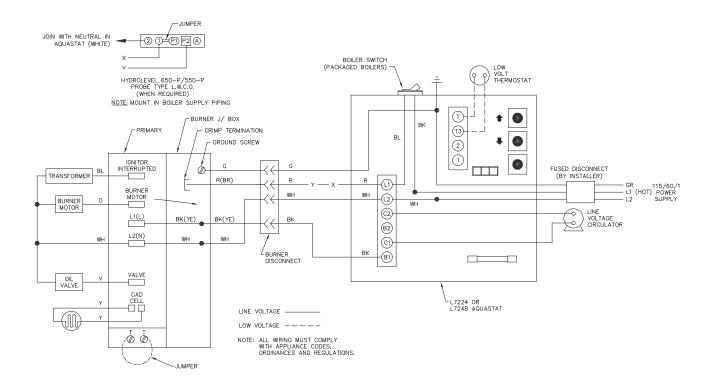
Figure 4.3: Water Boilers, Packaged
