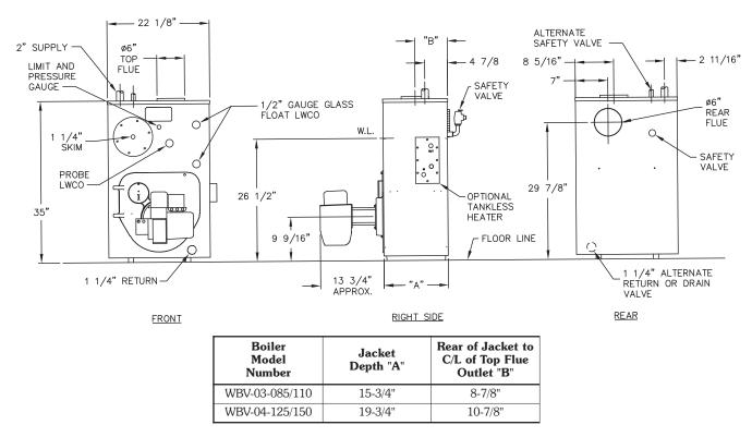
Figure 7.2: Boiler Dimensions, Steam Boiler
