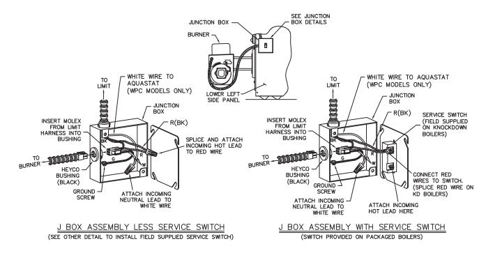
Figure 4.1: Junction Box Wiring, Steam and Knockdown Water Boilers
