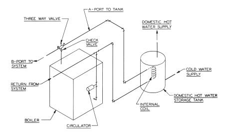
Figure 3.6: Piping with Peerless Indirect Water Tank
