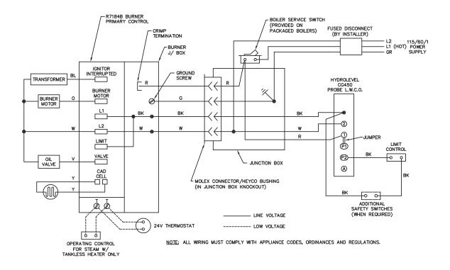
Figure 4.5: Steam with Probe Low Water Cut-off
