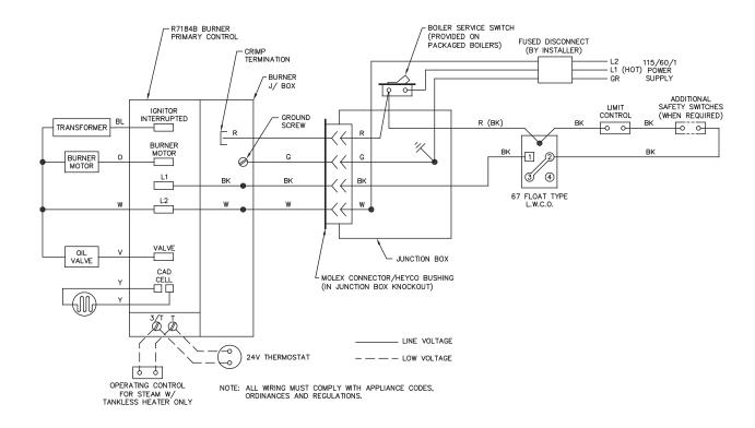
Figure 4.4: Steam with Float Low Water Cut-Off
