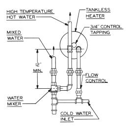
Figure 3.4: Tankless Coil Piping, Water Boiler
