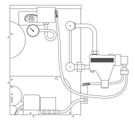
Figure 3.7: Float Low Water Cut-off
