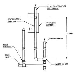
Figure 3.3: Tankless Coil Piping, Steam Boiler
