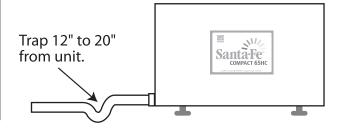
If floor drain is not easily accessible, a condensate pump kit with a 20' hose is available. Refer to page 5 for ordering accessories.
