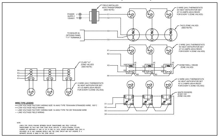
Figure IW-5: Multiple Zone System with Zone Valves
