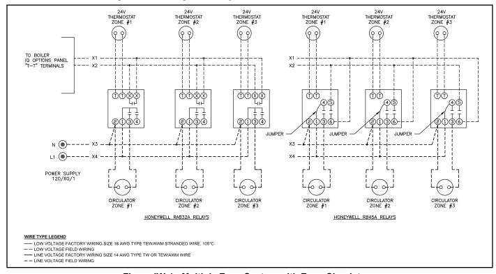
Figure IW-4: Multiple Zone System with Zone Circulators
