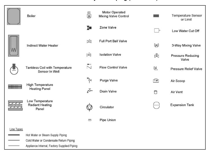
Figure D-0: Piping Schematic Symbols
