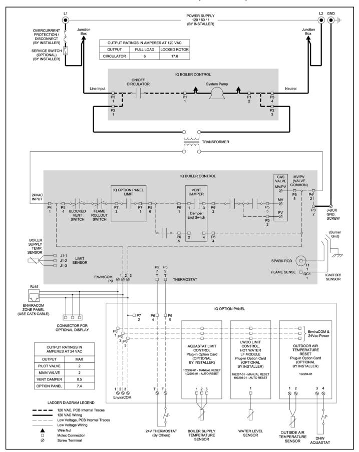
Figure IW-2: Wiring Schematic
