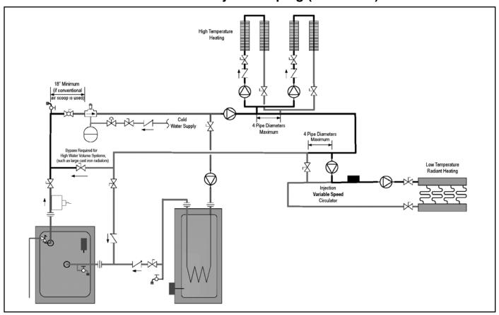
Figure D-W5: Water Boiler, Indirect Water Heater
