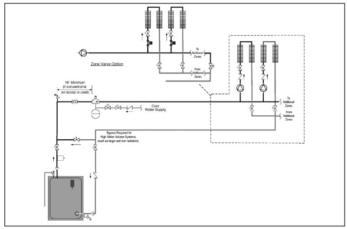
Figure D-W2: Water Boiler, Two or More Zones
