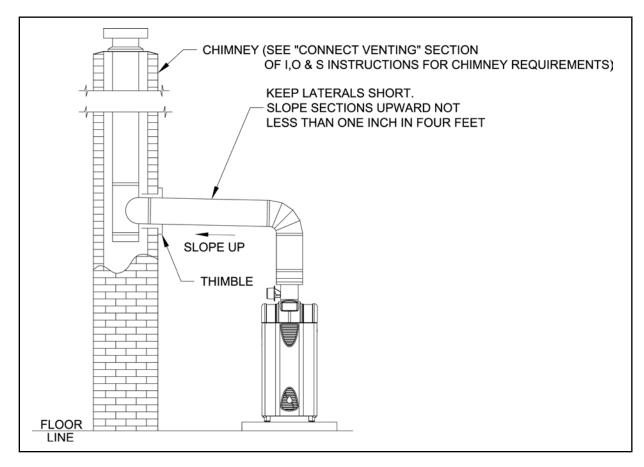
Figure B-1: Typical Atmospheric Vent Installation
