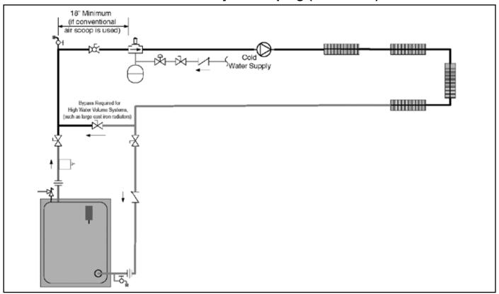
Figure D-W1: Water Boiler, Series Loop
