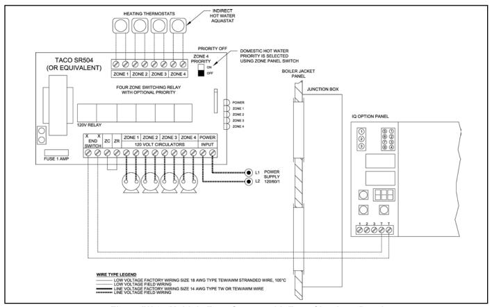
Figure IW-6: Multiple Zone System with Zone Circulator Panel
