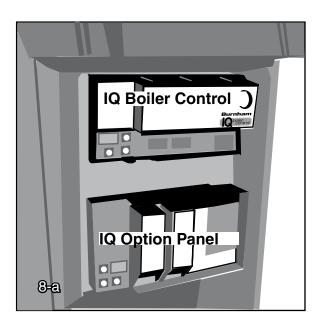
The IQ Boiler Control display, along with Up  $\, \hat{\mathcal{Q}} \,$ , Down  $\, \mathbb{Q} \,$ , and " $\, \mathbb{Z} \,$ " keys may be used to view boiler operating status (Figure 8-b). Please note that these keys look similar to the keys on the IQ Option Panel but are in a different orientation, and they perform different functions.
