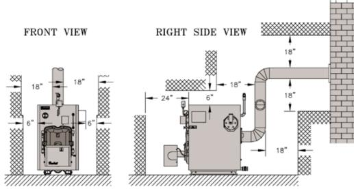
Figure 2: Minimum Installation Clearances To Combustible Materials (Inches)
