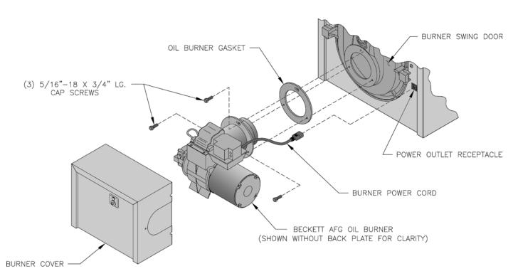
Figure 10: Oil Burner Installation
