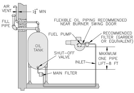
Figure 21: Single Pipe Oil Line
