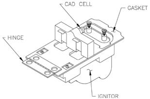
Figure 26: Cad Cell Location
