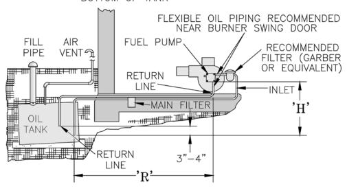
Figure 22: Two Pipe Oil Lines
