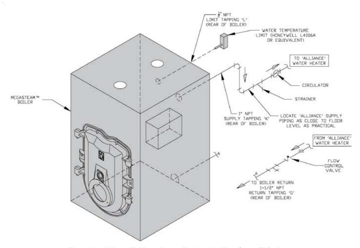
Figure 13: Alliance™ Water Heater Piping with MegaSteam™ Boiler
