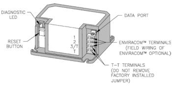
Figure 25: R7184 Terminals, LED and Reset Button
