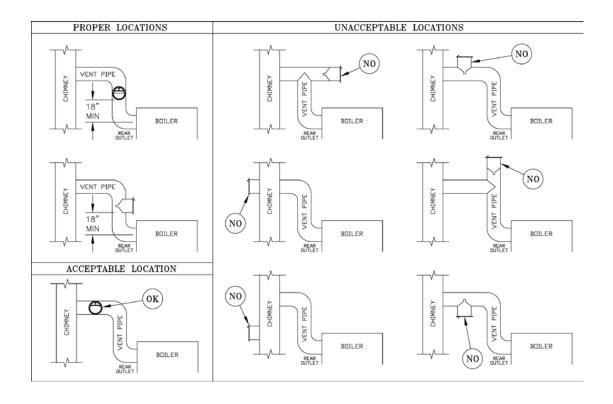
Figure 15: Proper and Improper Locations of Draft Regulator
