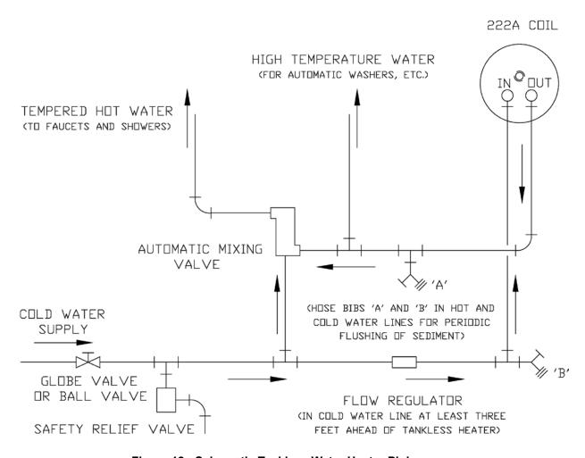
Figure 12: Schematic Tankless Water Heater Piping
