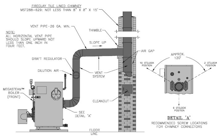
Figure 14: Recommended Vent Pipe Arrangement and Chimney Requirements
