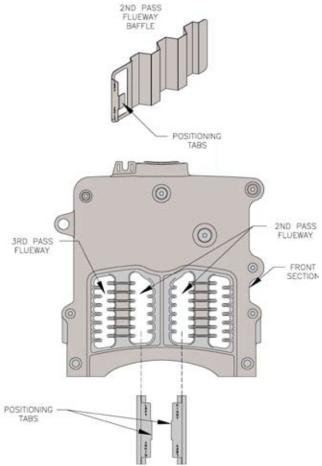
Figure 6: Flueway Baffle Positioning/Orientation in Flueways
