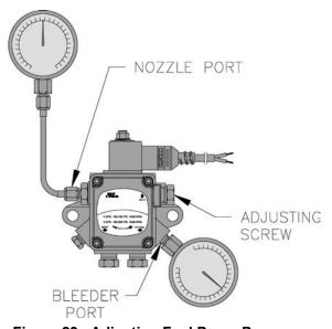
Figure 23: Adjusting Fuel Pump Pressure
