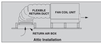
Same unit can be installed for horizontal or vertical supply air flow with simple field conversion.
