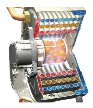
316L stainless steel full flow heat exchanger incorporating tri-parallel flow design that yields high efficiency through even heat transfer and low water pressure drops. This patented radial flow heat exchanger is manufactured using robotic laser welding techniques for precision construction. H stamp ASME code certified.
