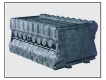
The cast iron sections of the Smith GV100 Series boiler have thicker walls and up to 30% more cast iron than competitive boilers. Extra-deep 2 3/4" sections increase the boiler's water content and total water surface. Benefits of these superior design features include better heat transfer and heat retention, and an Annual Fuel Utilization Efficiency exceeding 83%. The deeper section design also helps reduce mineral buildup and corrosion.
