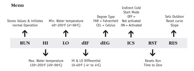
To start the control operation, you must return to RUN on the menu, and press Function. Normal operation will begin.
