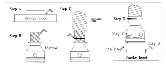
**NOTE:** - The adapters are multi-start, left hand thread, with one thread twice the width of the others. Therefore, care must be taken to ensure that the correct threads are engaged before tightening in a counter clockwise direction.
