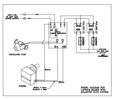
CAPRICE WIRING DIAGRAM FOR SENTRY 2100 (direct Vent)
