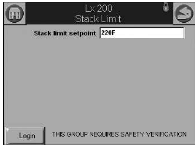
Figure 4-11 Stack Limit Screen
