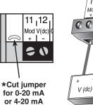
Connection to Operate Modulating Boiler
