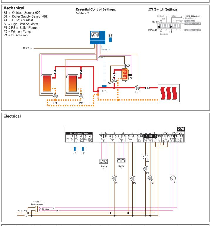
**System Description:** The Boiler Control 274 controls two On/Off boilers to provide DHW and outdoor reset operation for the space heating zones. The 274 receives a 0-10 V(dc) or 2-10 V(dc) signal from an EMS system which creates a target temperature for the control, which then stages the boilers as required. The 274 also controls a DHW pump. This system can provide DHW priority over space heating to provide faster DHW tank recovery.
