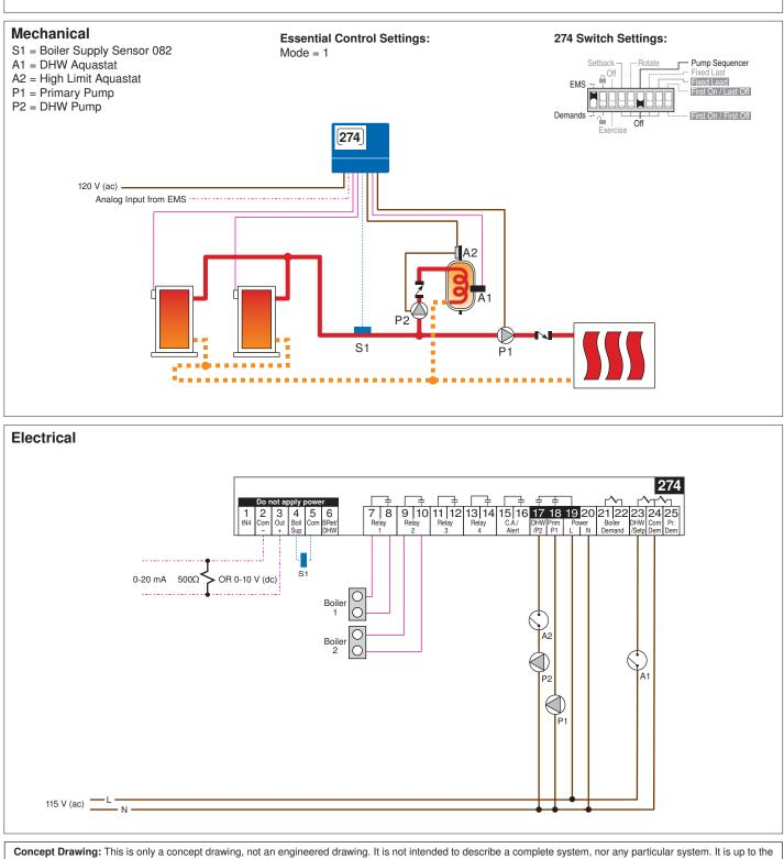
**System Description:** The Boiler Control 274 controls two, 2 stage boilers to provide DHW and outdoor reset for the space heating zones. The tN4 Gateway 483 allows for remote monitoring of the 274 and access to the tN4 system through a web browser. The 274 receives a boiler demand over the tN4 boiler bus from the tN4 thermostats. A 161 Setpoint control is used to create a DHW demand over the tN4 network. This allows for both DHW production and the use of the pump sequencer function.
