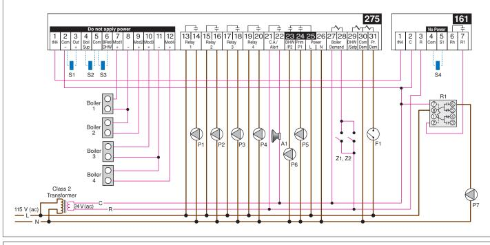
**System Description:** The Boiler Control 275 modulates up to four modulating boilers to provide DHW and outdoor reset for the space heating zones. The tN4 Gateway 483 allows for remote monitoring of the 275 and access to the tN4 system through a web browser. The boilers are piped in primary-secondary and the boiler pumps are controlled by the 275 to allow post purging of the boilers after they have shut off. The 275 receives a boiler demand over the tN4 boiler bus from the tN4 thermostats.
