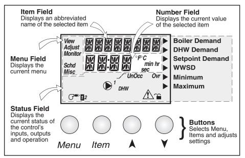
The tekmar Boiler Control 262 has a Liquid Crystal Display (LCD) and four push buttons (Menu, Item, A,∀) which are used to view and adjust the settings.
