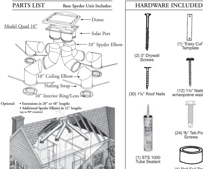
(1) "Easy Cut" Template (12) 13/4" Nails w/neoprene washer (24) 3/8" Tek-Point Screws (1) Roll Foil Tape
