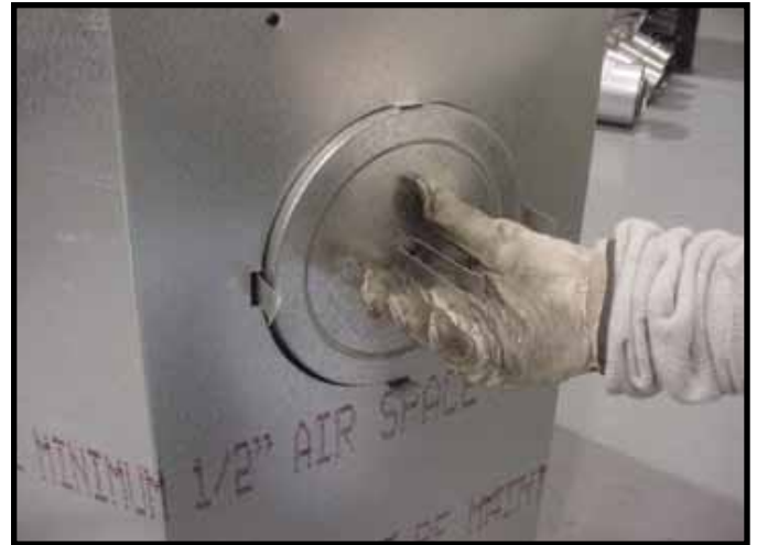
Figure 9.10 Fold the center parts of the retaining band out and use to remove the seal cap.
