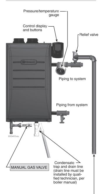
Relief valve drain line (must be run to safe . drainage location — must be installed by qualified technician, per boiler manual)
