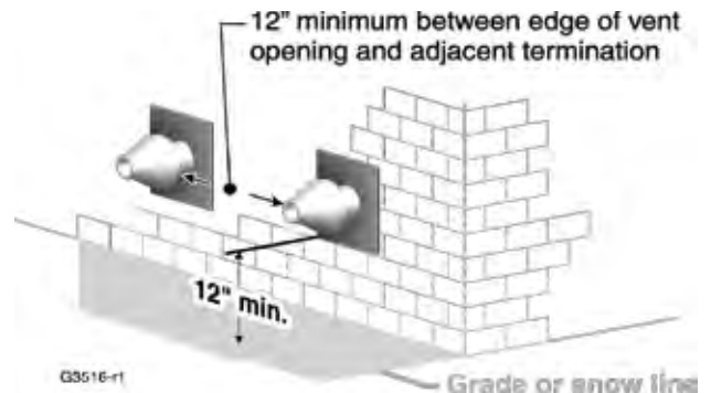
Figure 27 Termination location — concentric termination — multiple boilers — clearance from vent of one to air intake of the next
