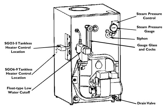
Steam Boiler Controls With Float-Type LWCO (Optional Tankless Heater Control) FIGURE 5
