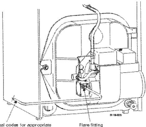
See local codes for appropriate arrangement and piping of filter, control valves, etc., back to oil tank.
