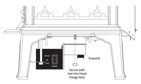
Figure 36. Attach Control Switch Box.
