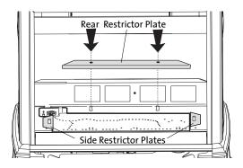
Figure 6. Installing the Air Intake Restrictor Plates.
