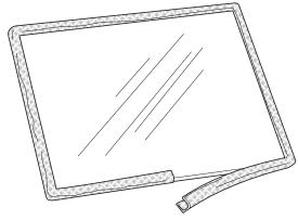
Figure 34. Wrap the gasket around the glass panel.
