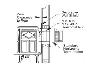
Figure 11. Min. / Max. Horizontal Run
