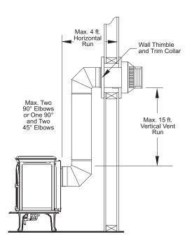
Figure 13. Horizontal Termination with Vertical Rise.
