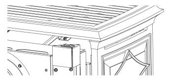
Figure 32. Burner Control Switch location.
