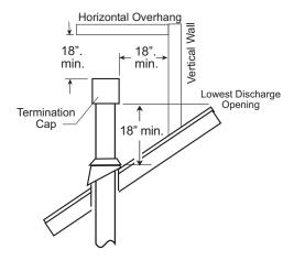
Figure 8. Minimum vertical termination height and roof clearance.
