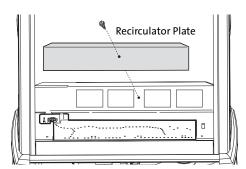
Figure 5. Remove Recirculator Plate.
