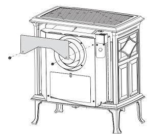
Figure 15. Wall Shield installation.
