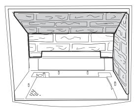
Figure 44. Install the Upper and Side Panels.
