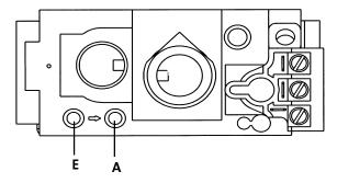
Figure 24. Pressure test points.
