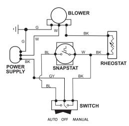
Figure 38. Blower Wiring Diagram
