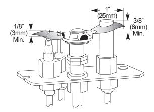
Figure 30. Proper pilot flame appearance.
