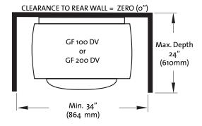
Figure 2. Alcove Installation Clearances.
