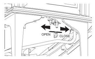
Figure 26. Air Shutter adjustment
