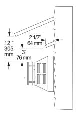
Figure 14. Termination Clearance to overhangs
