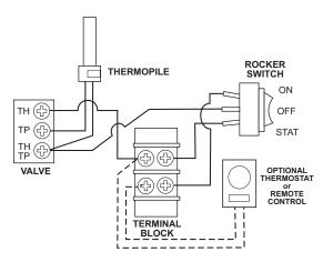
Figure 27. Accessory wiring diagram.
