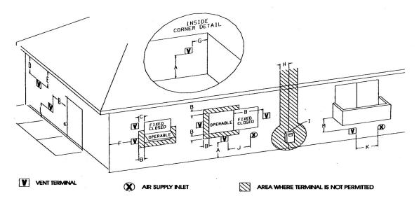
Figure 17. Vent Terminal Clearances - National Fuel Gas Code.
