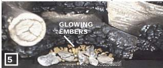
Randomly place the charcoal embers along the front of the support pan and some onto the screen in a realistic manner. Fine dust found in the bottom of the bag should not be used. Do not place any embers on the burner.
