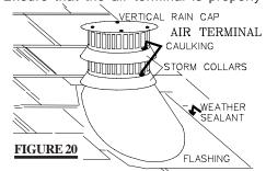
ing. Make weather-tight by sealing with caulking. Where possible, cover the sides and top edges of the flashing with roofing material.
