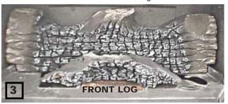
Set the two crossover logs into the pockets provided on both the front and rear logs., as shown.
