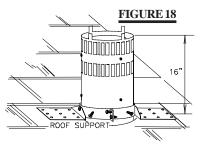
2. Slip a 4" diameter length of aluminium flexible liner a minimum of 2" over the inner sleeve of the air terminal.
