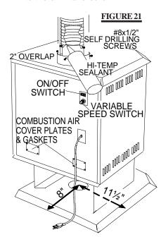
Ensure that the sealant is not visible on the exterior pipes once installation is completed. An optional decorative brass band is available for this use. (Standard with a GD175 kit). In the event that the venting must be disassembled, care must be taken to reseal the venting.
