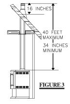
Deviation from the minimum vertical vent length can create difficulty in burner start-up and/or carboning.
