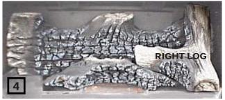
Tear the glowing embers into pieces and place onto the screen beneath the front log. Care should be taken to shred the embers into *thin, small irregular pieces* as only the exposed edges of the fibre hairs will glow when exposed to direct flame; however care should be taken to not block the burner ports. Blocked ports can cause an incorrect flame pattern, carbon deposits and delayed ignition.
