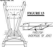
1. Determine the air terminal location and move the stove into position. Cut and frame 9 inch openings in the ceiling and the roof to provide the minimum 1 inch clearance between the stove pipe and any combustible material. Try to
