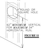
For optimum performance, the stove pipe should rise  $\frac{1}{2}$ " per foot of run.
