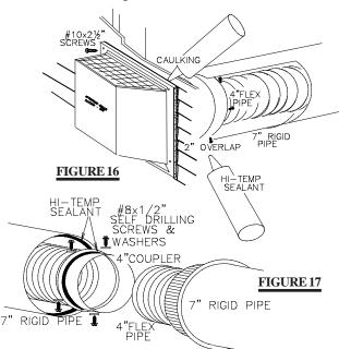
**4.** If more than one length of liner needs to be used to reach the stove, couple them together as illustrated in **FIGURE 17**. Seal the joints using the same procedure as described above.
