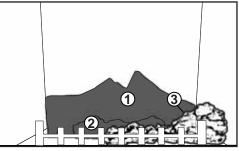
**6.1.3** Position the front right log just behind the grate lining up the holes in the bottom with the studs located on the log support.
