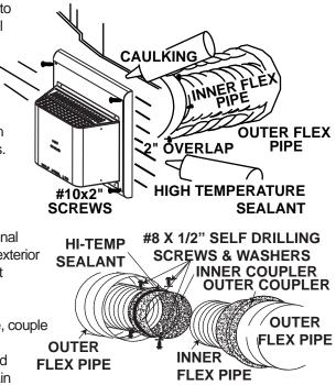
The air terminal mounting plate may be recessed into the exterior wall or siding no greater than the depth of its return flange. - 23.1
