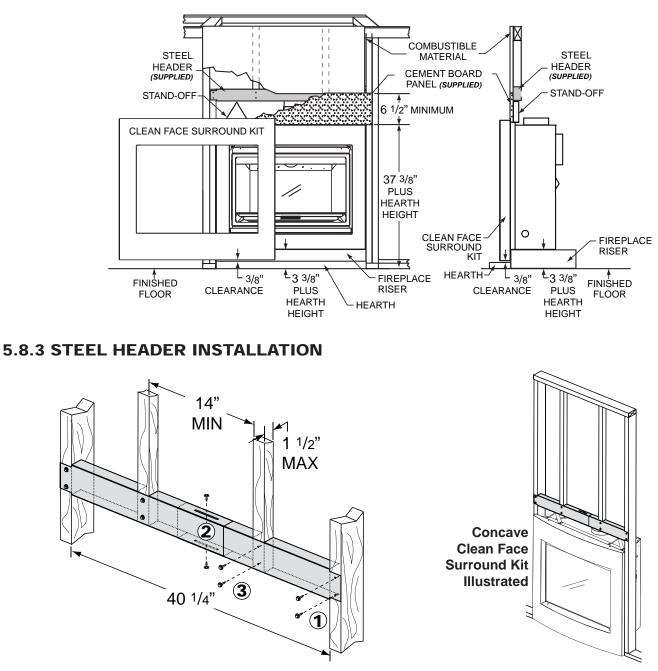
NOTE: The optional cleanface trim kit must be installed before proceeding.
