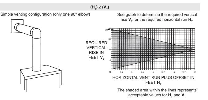
For vent configurations requiring more than one 90° elbow, the following formulas apply: Formula 1:  $H_T \leq V_T$
