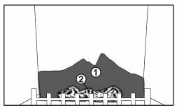
**6.1.2** Move the charcoal strip into position lining up the holes in the bottom with the studs located on the burner on the burner. Ensure strip sits flat on the burner.
