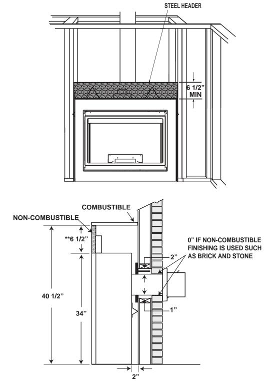
\*\* Installation requires a minimum 6 1/2" of non-combustible facing above the top of the appliance.
