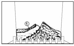
**6.1.1** Place the rear log so that it rests against the two log brackets on the back wall of the firebox. The air space between the log and firebox back is used to facilitate combustion air flow
