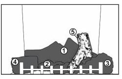
**6.1.5** Line up the square hole in the right crossover with the square post located on the right side of log and install as shown.
