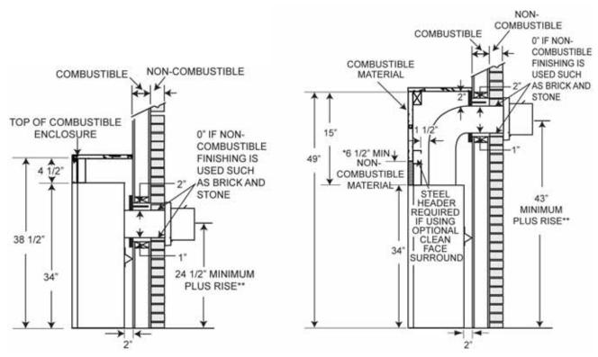
The appliance requires a minimum enclosure height of 38 1/2" (REAR VENT) 49" (TOP VENT). For temperature requirements, the enclosure space around and above the appliance must be left unobstructed.
