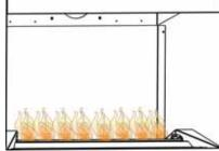
FLAME MUST ENVELOP UPPER 3/8" TO 1/2" OF FLAME SENSOR
