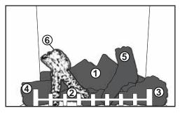
**6.1.6** Line up the rectangular hole in the left crossover with the rectangular post located on the left side of log and install as shown.
