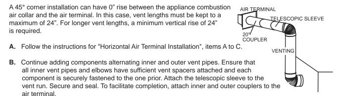
**C.** Install the air terminal. See item 3 of the Horizontal Air Terminal Installation. Extend the outer telescopic sleeve; connect to the air terminal assembly. Fasten with self tapping screws and seal.
