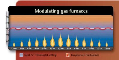
The Luxaire<sup>®</sup> Acclimate<sup>™</sup> modulating gas furnace has been designed to maintain your ideal temperature by modulating in one-percent increments. Comfort is dramatically increased as the furnace adjusts its level of operation up or down to offset the rate at which heat leaves your home.
