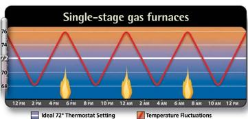
Traditional single-stage gas furnaces operate much like a light bulb—either on or off. This can create wide and uncomfortable temperature fluctuations in your home.
