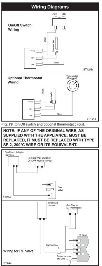
Fig. 80 Draft hood adapter wiring. 20012734
