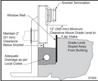
Fig. 39 Below grade installation.
