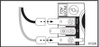
Fig. 51 Attach switch wires to valve.
