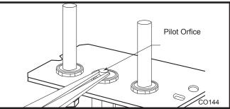
Fig. 70 Remove pilot orifice.
