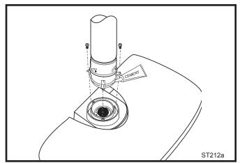
Fig. 19 Attach inner assembly to flue collar.
