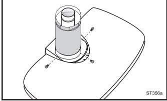
Fig. 22 Simpson Dura-Vent - install outer adapter pipe.
