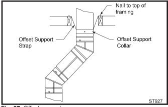
Fig. 37 Offset support. Supporting DIRECT-TEMP: Horizontal Support
