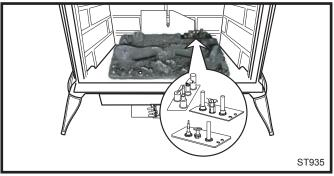
Fig. 53 Pilot assembly location.
