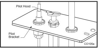
Fig. 67 Remove pilot hood.
