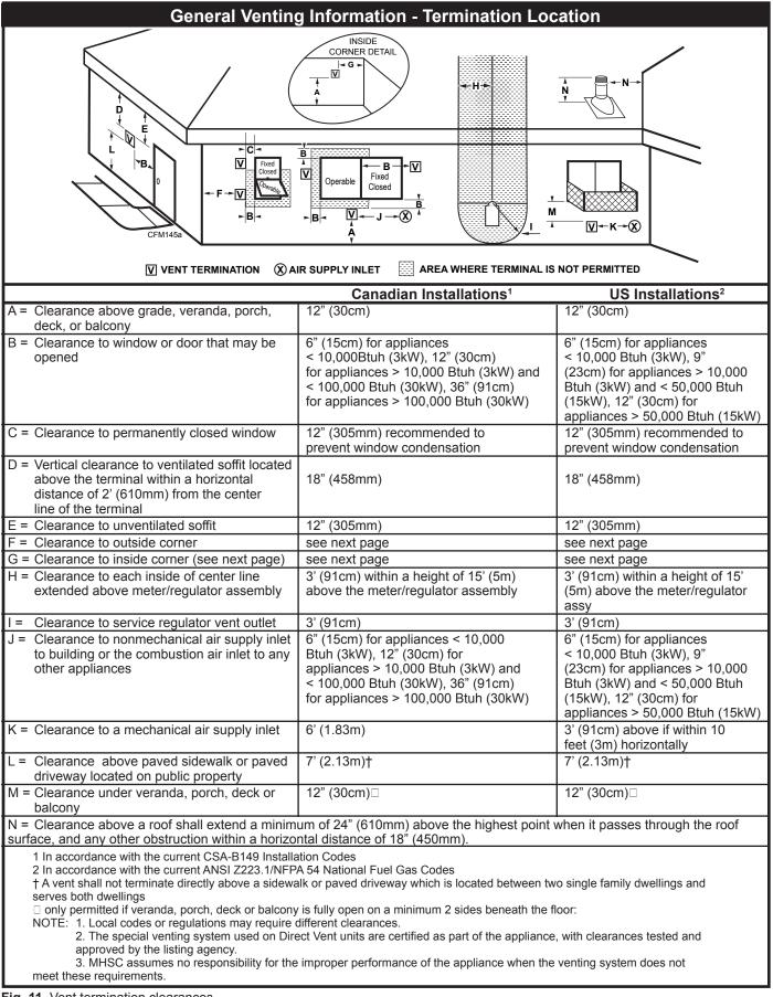
Fig. 11 Vent termination clearances.
