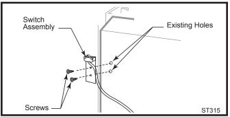
Fig. 50 Attach switch assembly to rear shroud.
