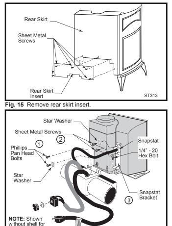
clarification **Fig. 16** Attach the fan assembly and the snapstat.
