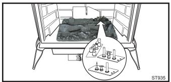
Fig. 66 Pilot assembly location.
