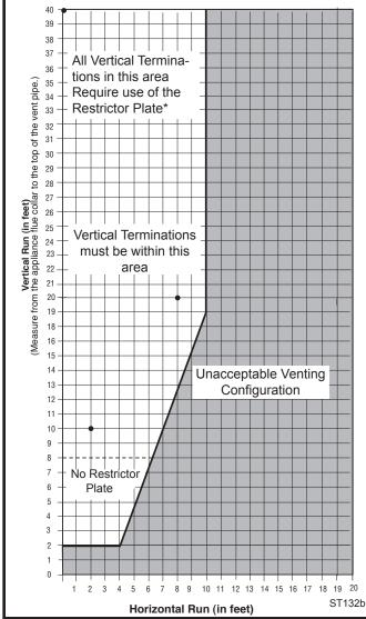
Fig. 8 Vertical vent termination window.
