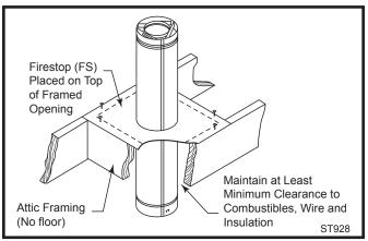
Fig. 38 Firestop spacer.
