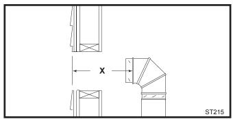
Fig. 26 Measure the horizontal length.
