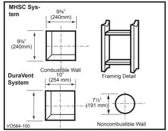
Fig. 23 Locate vent opening.
