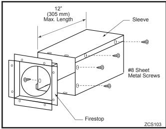
Fig. 24 Assemble the wall sleeve and firestop.
