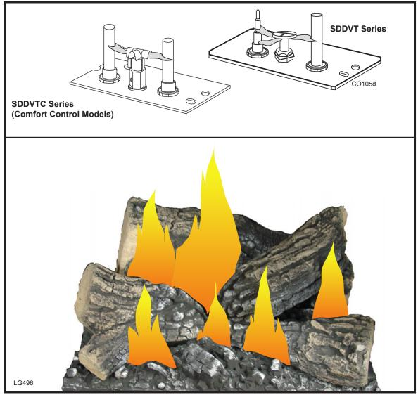
Fig. 55 Correct pilot and burner flame patterns.
