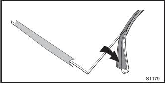
**Fig. 77** Wrap the gasket material around the outside iedge of the glass.
