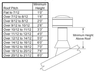
Fig. 44 Minimum Height Above Roof Requirements
