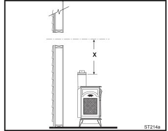
Fig. 25 Determine the vertical pipe length.
