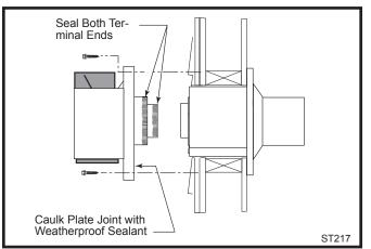
Fig. 28 Install the vent terminal.
