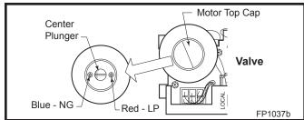
Fig. 65 Depress and turn center plunger.
