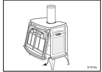
Fig. 75 Remove the stove front.
