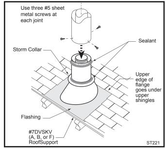
Fig. 32 Roof support and flashing.
