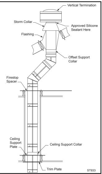
Fig. 43 Typical vertical venting configuration.
