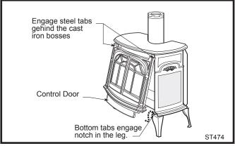
Fig. 52 Install the front plate.
