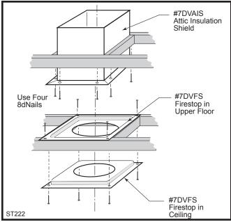
Fig. 31 Install firestops and attic insulation shield.
