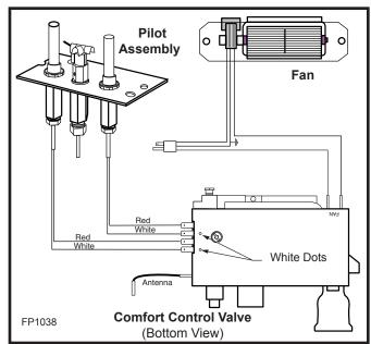
Fig. 58 Comfort valve wiring diagram.
