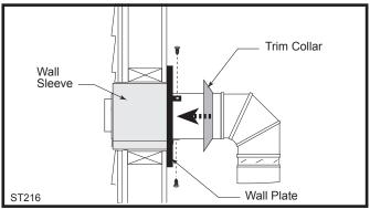
Fig. 27 Install the horizontal pipe and wall plate parts.
