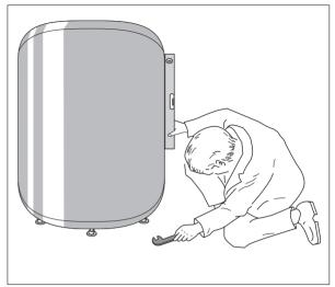
Fig. 5 Adjusting tank leveling bolts (sample picture)
