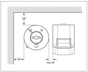
Fig. 1 Recommended clearance for installation and maintenance.
