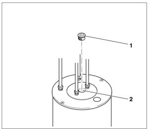
Fig. 11 Removal of inspection plug
