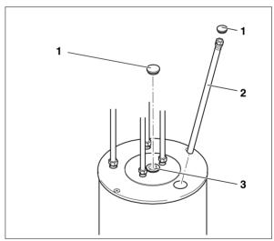
Fig. 10 Removal of magnesium anode rod
