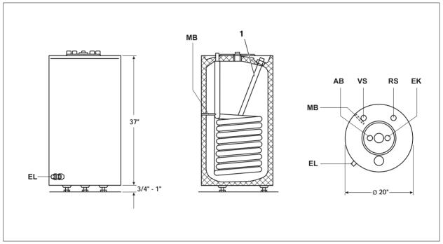
Fig. 4 Dimensions and piping connections (measurements in inches)
