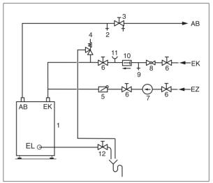
Fig. 6 Tank piping installation (sample picture)
