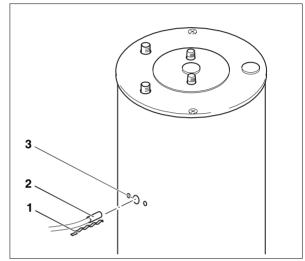
Fig. 7 Installation of temperature sensor
