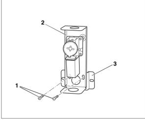
Fig. 8 Attaching bracket to aquastat
