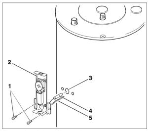
Fig. 9 Installation of Honeywell aquastat
