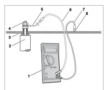
Fig. 15 Checking anode with multimeter
