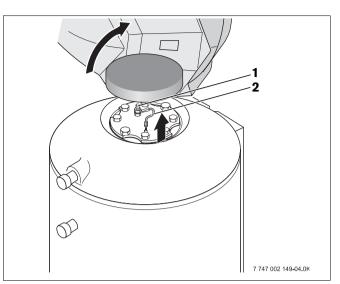
Fig. 7 Checking the magnesium anode connection
