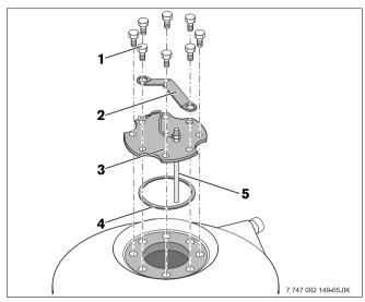
Fig. 17 Installing access port cover
