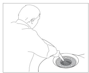
Hosing down the inside of the DHW tank Fig. 14
