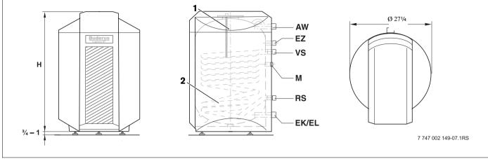
Fig. 2 Dimensions and connections (dim. in inches)
