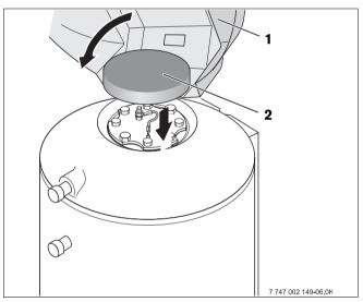
Fig. 18 Fitting the casing
