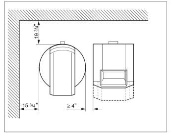
Fig. 4 Positioning the DHW tank (general layout)
