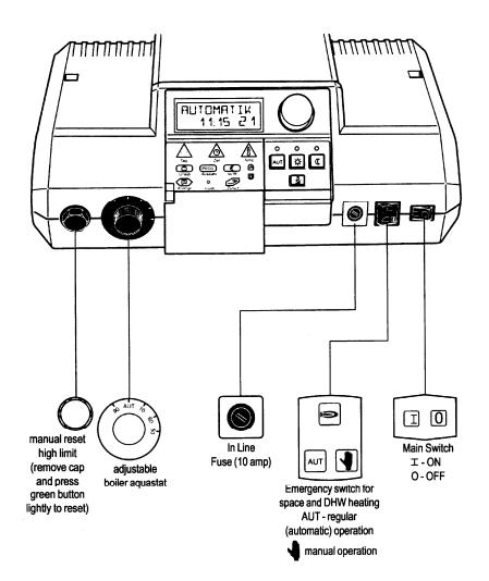
Note: When the emergency switch is in manual mode, set the adjustable boiler aquastat to 140°F or less. Risk of scalding! 4
