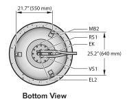
MB1 DHW Sensor LocationMB2 Solar Sensor Location
