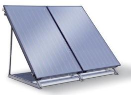
The Flat Roof Mounting Systems is compatible with both SKN and SKS collectors. The inclination can be easily adjusted to optimize your solar gain. Properly installed, the mounting system can withstand hurricane force winds and up to 35 lbs/ft<sup>2</sup> snow loads.
