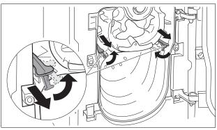
Fig.43 Adjusting the flue baffles
