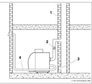
Fig. 12 Masonry chimney installation
