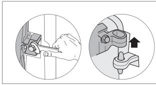
Fig. 4 Removal of burner door
