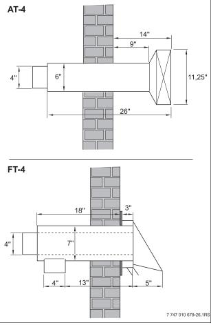
Fig. 15 Aerocowl (AT-4) and Concentric (FT-4) termination
