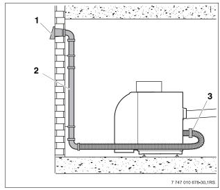
Fig. 20 Combustion air supply system
