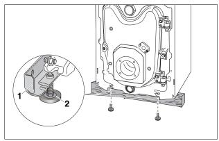
Fig. 10 Installation of boiler feet
