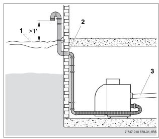
Fig. 21 Outside air intake riser
