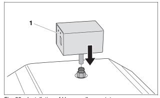
Fig. 29 Installation of Honeywell aquastat
