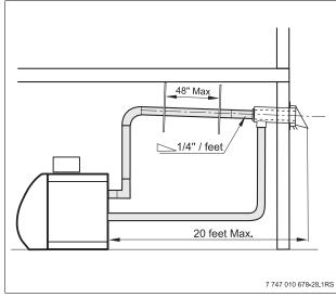
Fig. 18 Combination air intake/exhaust termination (Part No. FT-4)
