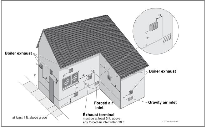
Fig. 16 Minimum clearance for termination
