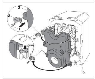
Fig. 9 Reversing burner door (on burner door)
