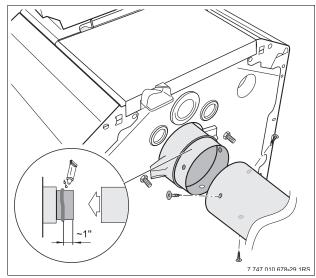
Fig. 19 Boiler exhaust pipe
