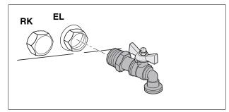
Fig. 24 Boiler Drain installation
