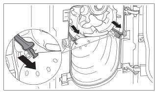
Fig.44 Removal of the flue baffles
