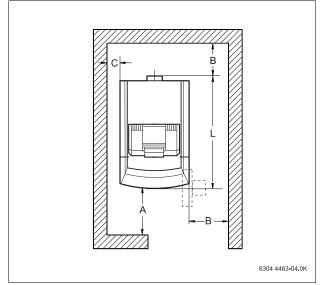
Fig. 7 Clearance dimensions for G125 boilers
