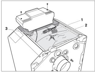
Fig. 34 Routing and connecting of capillary, sensor and electrical wiring
