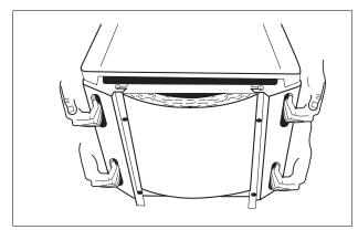
Fig. 5 Lifting and carrying the boiler
