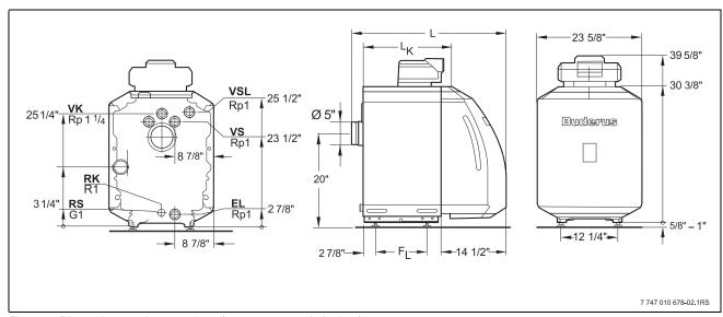
Fig. 2 Dimensions and connections (measurements in inches)
