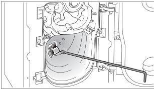
Brushing out the combustion chamber
