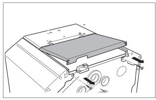
Fig. 28 Top rear cover removal
