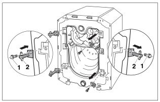
Fig. 8 Reversing burner door (boiler block)
