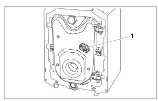
Fig.42 Pressure test port on burner door
