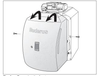
Fig. 3 Removing the front cover
