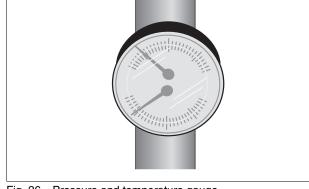
Fig. 26 Pressure and temperature gauge
