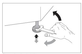
Fig. 11 Leveling the boiler
