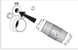
Fig. 22 Measuring thread length on 1-1/4" conversion nipple
