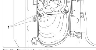
Fig. 50 Opening of burner door
