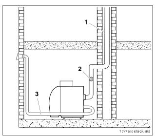
Fig. 13 5" Chimney liner installation
