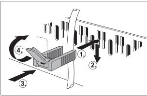
Fig. 36 Secure wiring with cable clips
