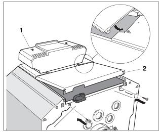
Fig. 37 Installation of rear top cover
