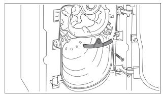
Fig.46 Removal of flue blocking plate
