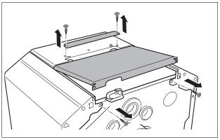
Fig. 30 Removal of rear top cover and top cover plate
