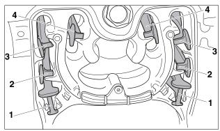
Fig.40 Blue baffle plates for fresh air operation
