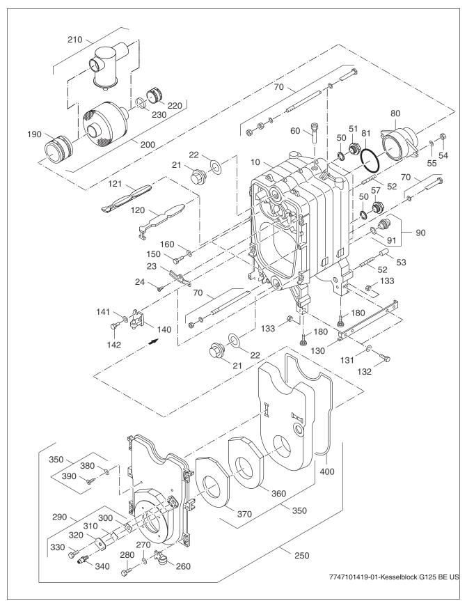
Fig. 60 Boiler block and burner door
