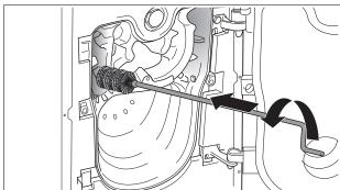
Fig. 51 Brushing out of flue passages
