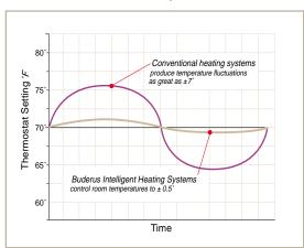
Conventional boilers leave room temperatures too hot or too cold—often varying up to  $\pm 7^\circ$  from the thermostat setting. Buderus low-temperature boilers provide more consistent heat, eliminating these wide temperature swings.
