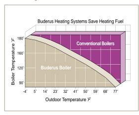
The difference between the constant high operating temperature of conventional boilers (typically 180°F) and the optimized water temperatures of a Buderus boiler means significant fuel savings.
