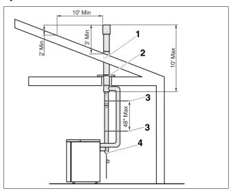
Fig. 25 Vertical flue system
