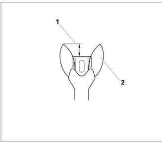
Fig. 41 Correct pilot flame setting
