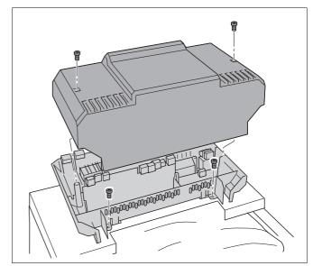
Fig. 14 Installation of Logamatic 2107 control
