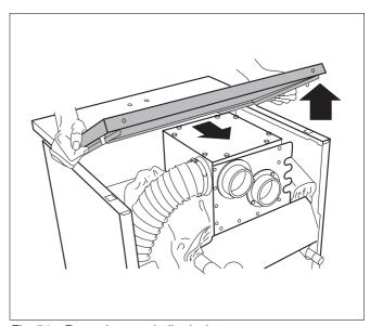
Fig. 51 Removing rear boiler jacket
