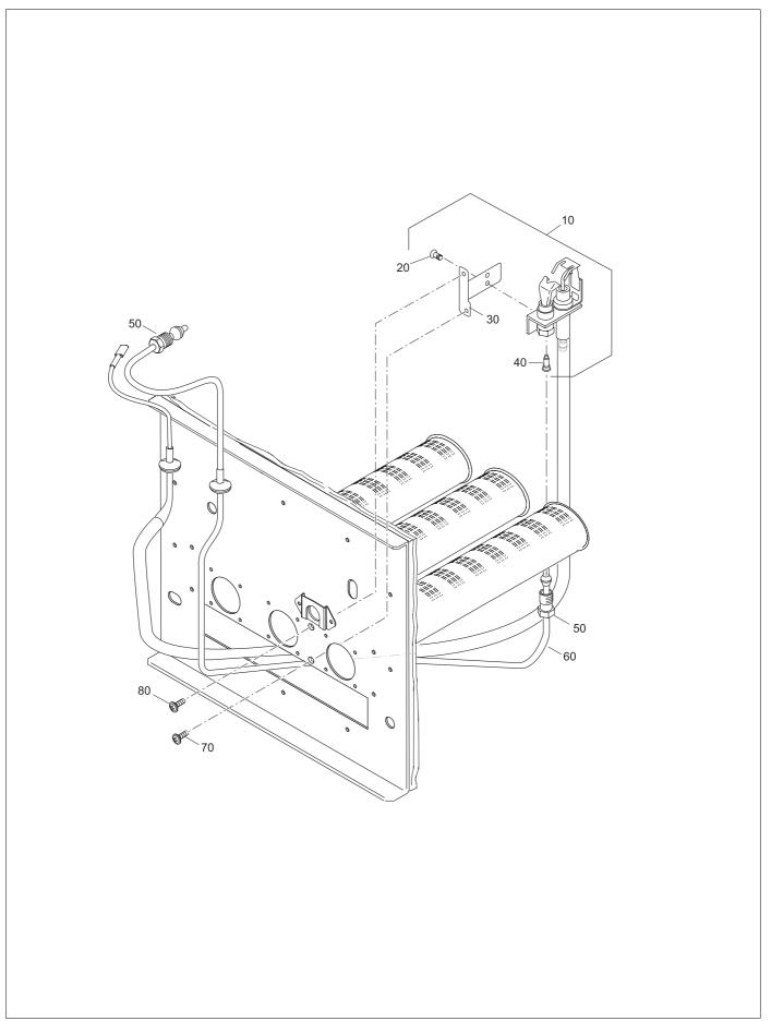
Fig. 62 Ignition burner
