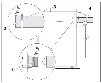
Fig. 26 Condensation trap
