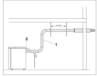
Fig. 32 Horizontal flue system using room air
