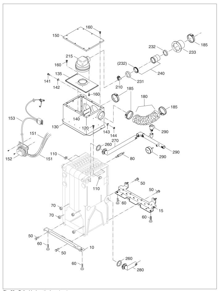
Fig. 58 Boiler block – attachment parts
