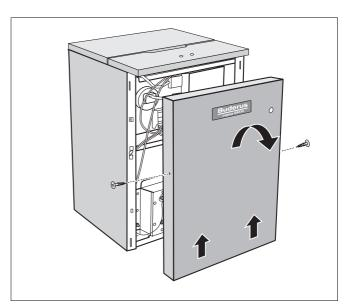
Fig. 11 Removing front panel of boiler
