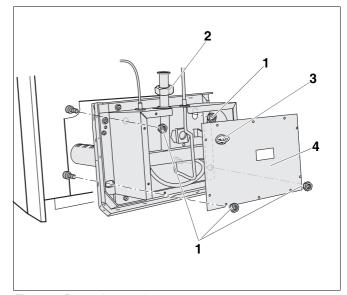
Fig. 50 Removing gas burner
