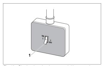
Fig. 46 Shutting down heating system (with aquastat)
