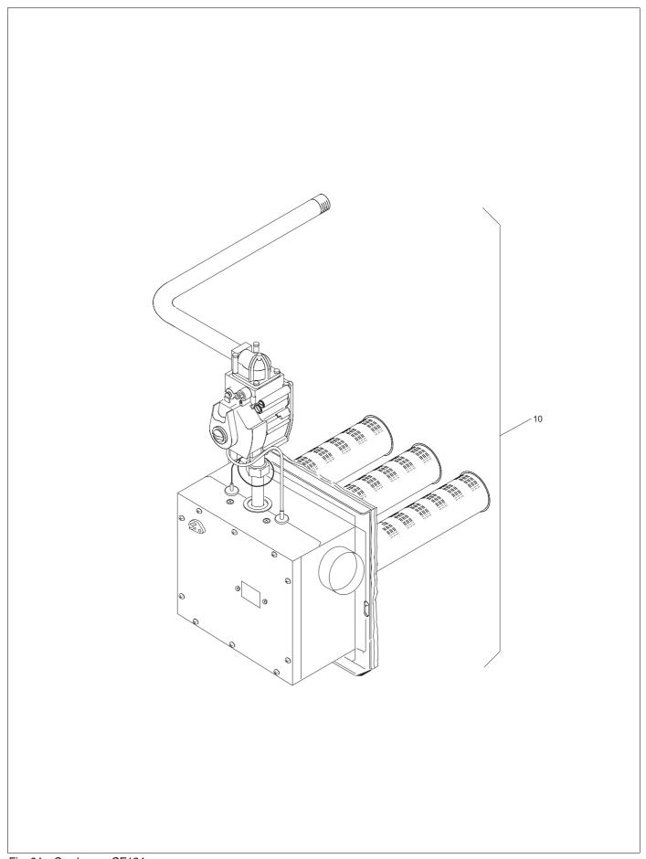
Fig. 64 Gas burner CE124
