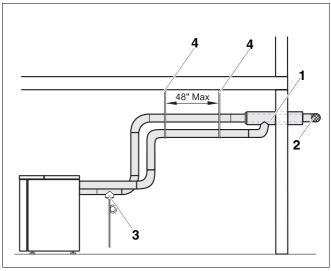
Fig. 28 Horizontal flue system
