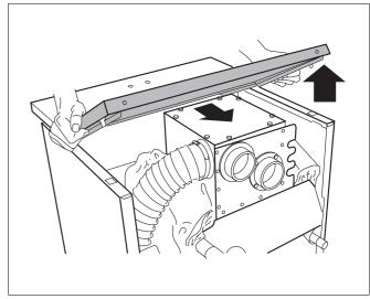
Fig. 12 Removing boiler jacket
