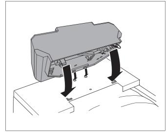
Fig. 13 Removing terminal cover
