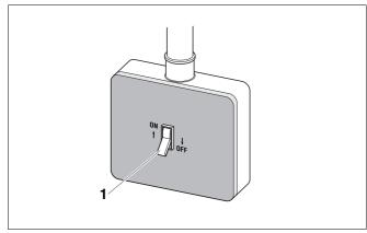
Fig. 37 Switching on heating system (with aquastat)
