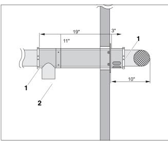
Fig. 23 Position of termination tee on the flue pipe
