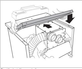
Fig. 19 Installing rear boiler cover
