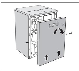
Fig. 35 Removing front panel of boiler
