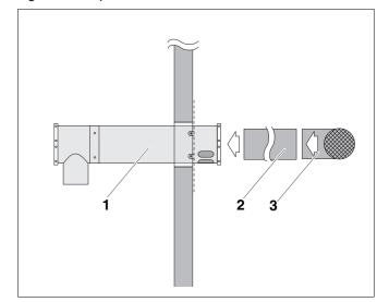
Fig. 22 Installing flue pipe
