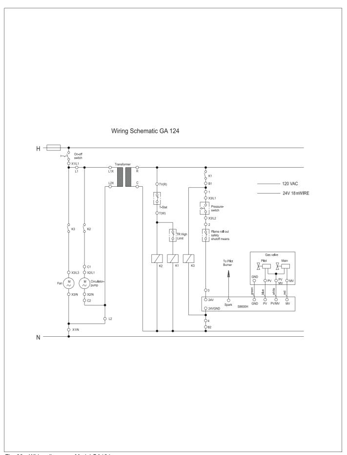
Fig. 66 Wiring diagram – Model GA124
