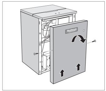
Fig. 44 Remove front panel of boiler
