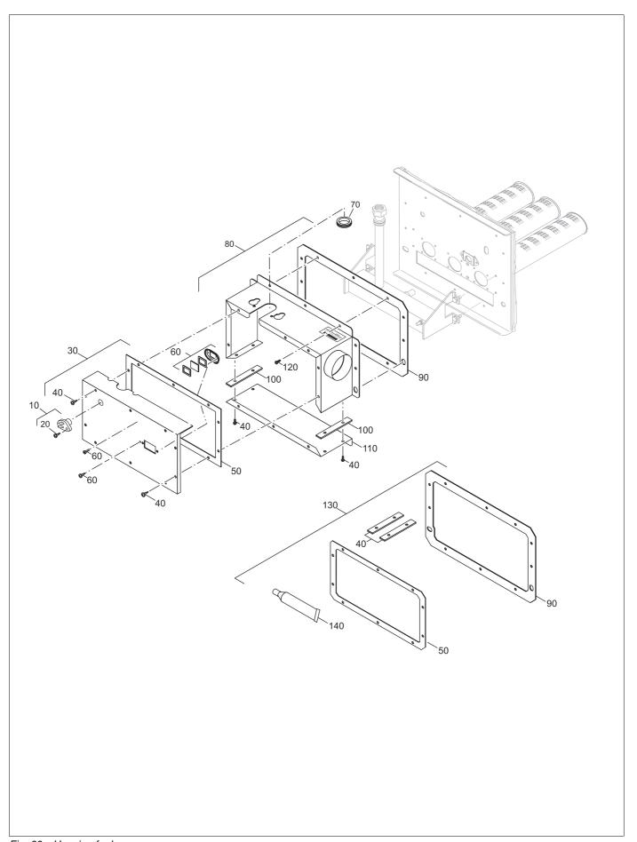
Fig. 60 Housing for burner
