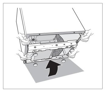
Fig. 8 Unscrewing screw-in feet
