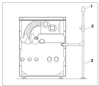
Fig. 20 Pipe connection to gas fittings - back view
