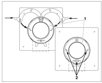
Fig. 24 Securing clips
