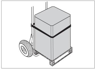
Fig. 4 Moving boiler with trolley
