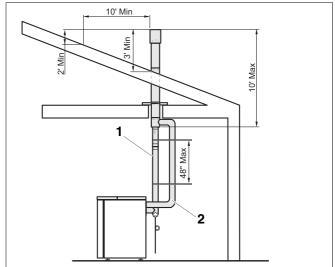
Fig. 33 Vertical flue system independent of room air
