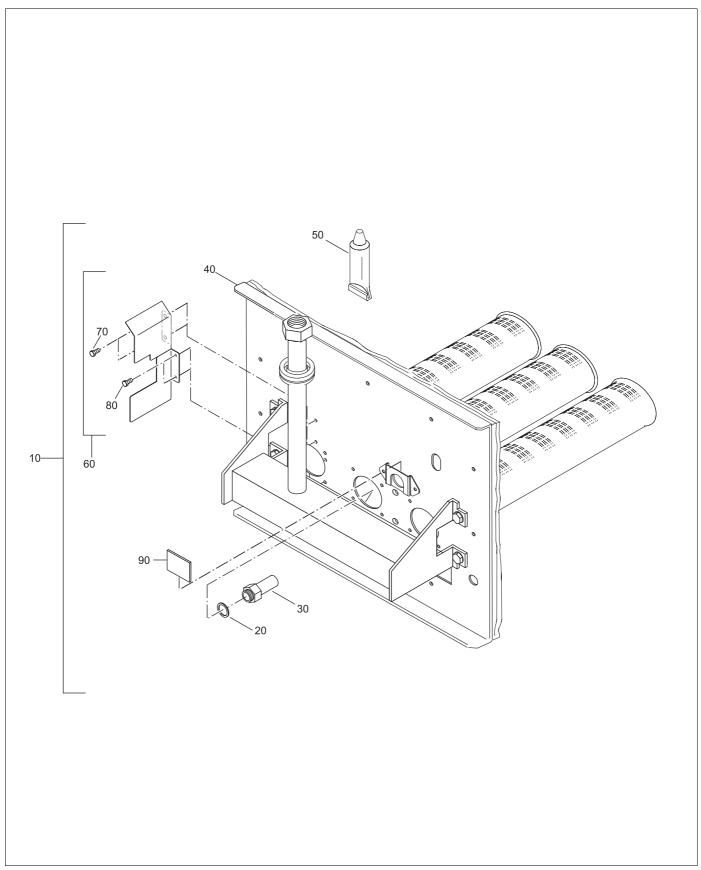
Fig. 63 Burner grate
