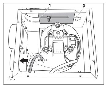
Fig. 30 Adjusting the combustion air baffle
