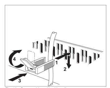
Fig. 16 Secure wiring with wiring clip
