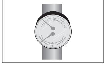
Fig. 34 Temperature/pressure gauge
